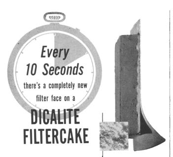
For all practical purposes, that means that you have a continuously fresh filtering surface—all the time—for consistent clarity and constant flow rate. The mechanism of this is simple. The particles of Dicalite filteraid added to the raw liquor as
